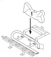
Figure 44 - Installing Log No. 1
